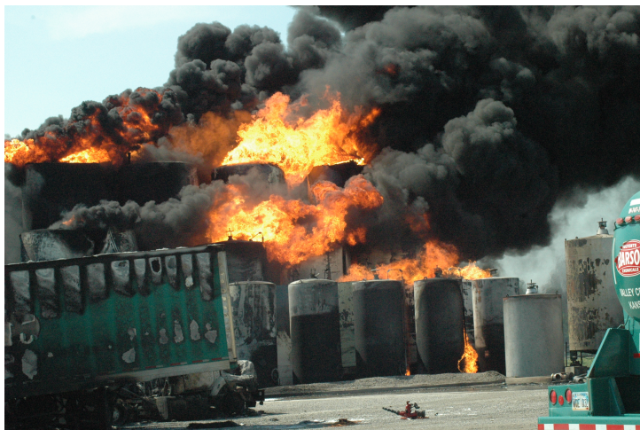
Figure 1.6: Static spark explosion of a chemical facility at Valley Center (Kansas, USA) in 2007 during a tank filling operation [34].
