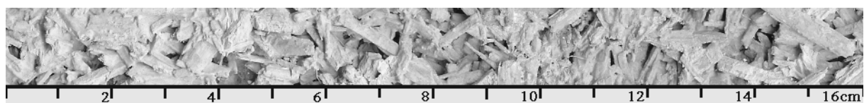
Figure 2: Macroscopic porosity of lime and hemp concrete – “wall” mixture
