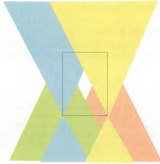
Figure 3.8: Bounded orientation angles impose the ICR to live outside a X-area or inside a diamond ace area
