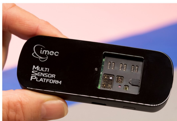
Figure 6: The ultimate output of the MSP-project - a wearable wristband device with integrated multi-sensor system.
