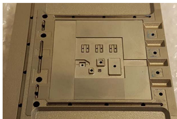
Figure 2: Tool employed for overmolding the MSP-demonstrator system.
