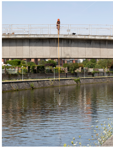
Figure 6. Radar system with a log-periodic antenna held at several distances from a water plane to determine the antenna characteristic functions R_i(\omega) , T(\omega) , and R_s(\omega) (antenna calibration). The radar measurements were performed in the 80–1000 MHz frequency range.
