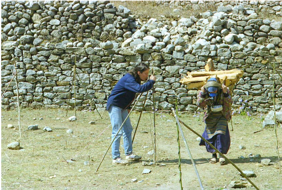
picture 9: Female Nepalese porter carrying a load equal to 75% of her body weight around the track where we made the oxygen consumption measurements. B. Schepens is adjusting the photocells that are used for controlling the walking speed. The Nepali are of small stature compared to Western subjects; yet they carry much heavier loads.
