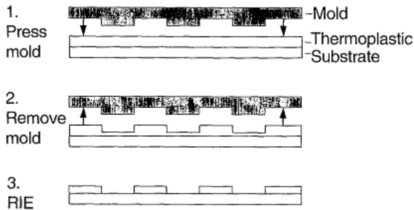
Figure 1.27 – Thermo-based nanoimprint lithography process, as described by Chou et al. A thermoplastic resist is spin-coated on the substrate to act as a mask, and a mold is pressed onto the mask to transfer the pattern. The mold is then removed, and a reactive-ion-etching (RIE) step is added to remove residual resist to expose bare substrate in the patterned regions [209].
