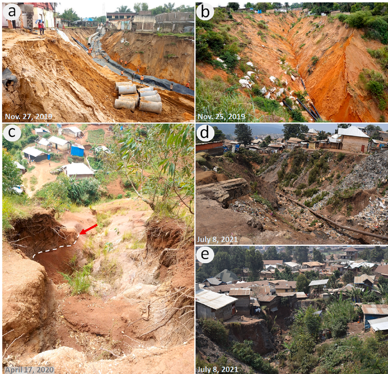
Fig. 2. Terrestrial photos of some of the urban gullies selected for this research in Kinshasa (a, b) and Bukavu (c, d, e). The locations of these photos is indicated in Fig. 1. Note the contrast in soil type and resulting gully morphology. Gullies in Kinshasa incise loose, largely homogeneous sandy soils, resulting in wide gully channels. Soils in Bukavu are clayey and more cohesive, often resulting in a more narrow gully channels. The red arrow in (c) indicates a reddish paleosol separating a relatively recent volcanic outflow from a clay soil below it, which resulted from the alteration of an older lava layer. (For interpretation of the references to colour in this figure legend, the reader is referred to the web version of this article.)
