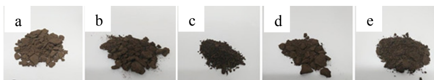
Figure 1. Biochars on a temperature of 160 (a), 180 (b), 200 (c), 220 (d), 240 (e)°C with residence time of 4 hours.
