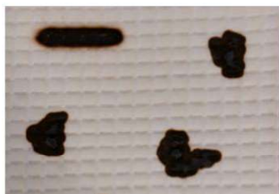
Figure 3: Results from the flame-retardant results (according to standard BS 7175 test) for a) the 30 wt% and b) 15 wt% application level of the novel phosphorylated dendroketol 'P-dendroketol, c) compared to the commercially available 'Ecoflam' flame retardant of Devan as reference. Both application levels of the novel bio-based flame retardant report a 'pass' rating after extinguishing a flame induced by a 35 mm torch, identical to the commercial flame-retardant.
