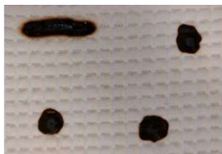
Figure 3: Results from the flame-retardant results (according to standard BS 7175 test) for a) the 30 wt% and b) 15 wt% application level of the novel phosphorylated dendroketol 'P-dendroketol, c) compared to the commercially available 'Ecoflam' flame retardant of Devan as reference. Both application levels of the novel bio-based flame retardant report a 'pass' rating after extinguishing a flame induced by a 35 mm torch, identical to the commercial flame-retardant.
