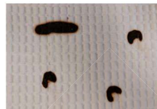
Figure 3: Results from the flame-retardant results (according to standard BS 7175 test) for a) the 30 wt% and b) 15 wt% application level of the novel phosphorylated dendroketol 'P-dendroketol, c) compared to the commercially available 'Ecoflam' flame retardant of Devan as reference. Both application levels of the novel bio-based flame retardant report a 'pass' rating after extinguishing a flame induced by a 35 mm torch, identical to the commercial flame-retardant.
