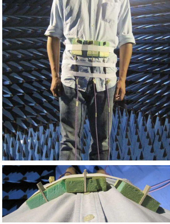
Figure 3.6: Position and polarization of the folded dipole antennas on the trunk in \vec{\rho} -polarized scenarios. The antennas were fixed by green foam blocks.
