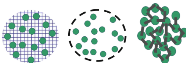
Figure I.5 - Protein immobilization strategies: (a) entrapment, (b) encapsulation, (c) and self-immobilization. Proteins are represented by circles. Adapted from Braddy et al. with permission from Springer Nature. 27
