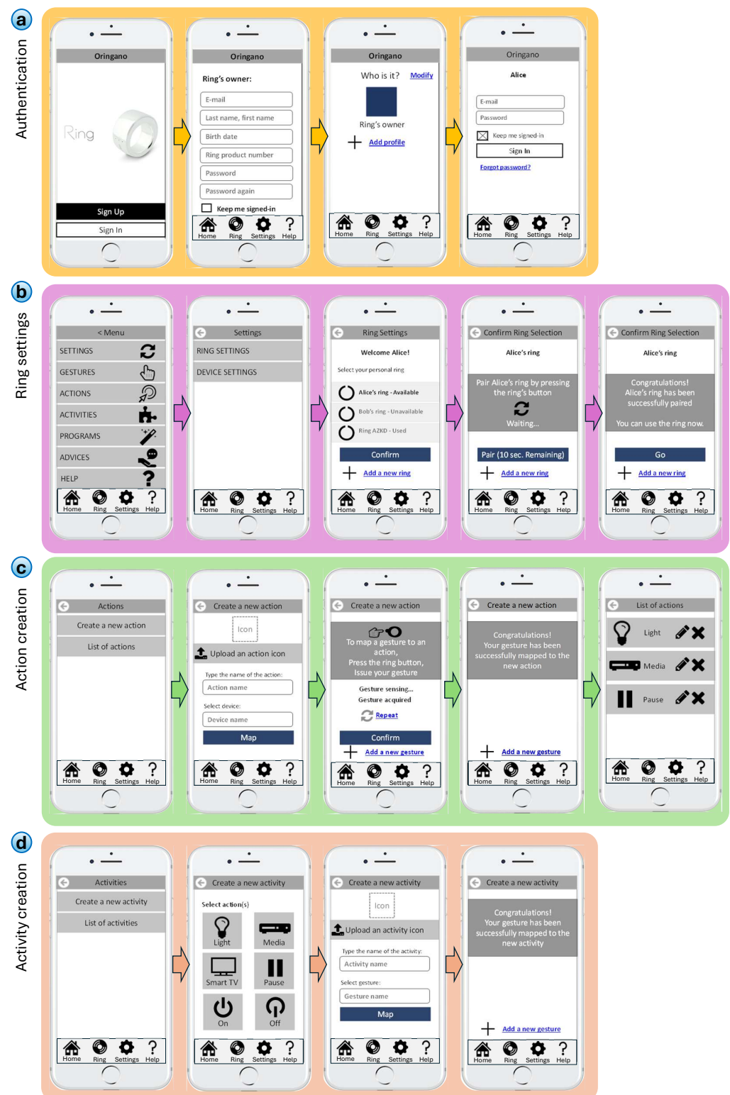
Figure A5. Interaction map of ORINGANO: (a) Authentication or sign in to the app. (b) Configure, list, Smart Ring Association by user's profile. (c) Action creation or view the list of actions, such as "Turn on light". (d) An activity allows you to trigger a sequence of actions.
