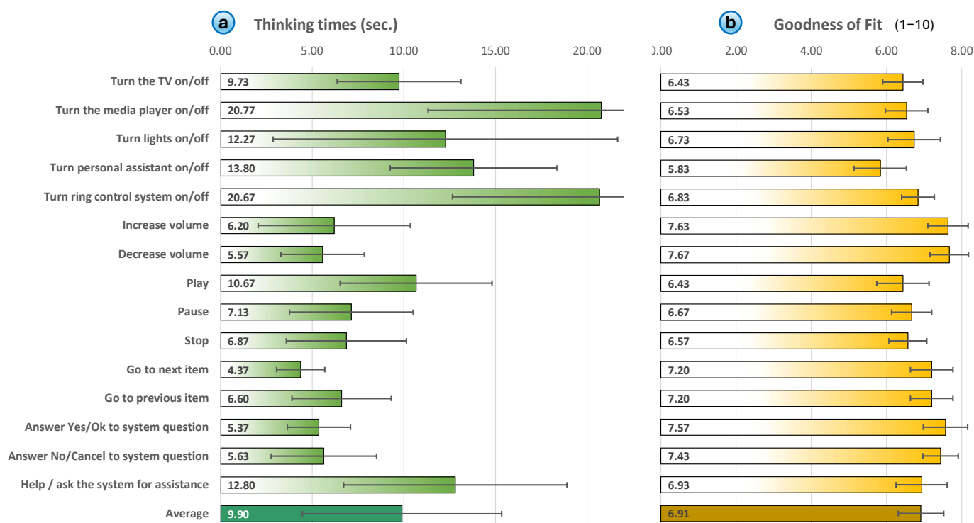
Figure 10. THINKING TIMES (a) and GOODNESS OF FIT (b) of shared ring-based gestures proposed for each referent. Error bars show a confidence interval of 95%.
