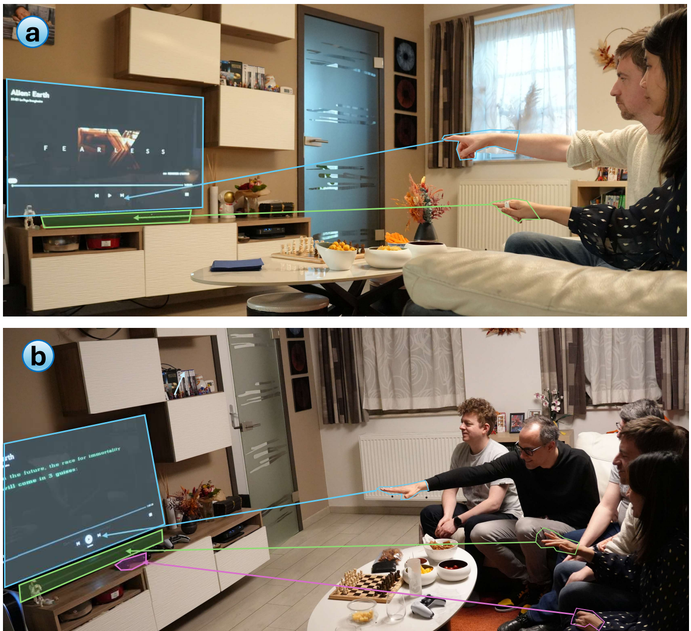
Figure 1. Ring-based gestures shared among users with ORINGANO: (a) A user advances through a movie by pointing the smart ring (in blue) to a smart TV and moving it to the right; a second user increases the volume by pointing the smart ring (in green) to a sound bar and rolling it clockwise. (b) A user switches the subwoofer on by pressing the ring to it (in purple), while a second user plays the current movie by selecting the smart ring to play (in blue), and a third user decreases the volume by rolling the smart ring counterclockwise (in green).
