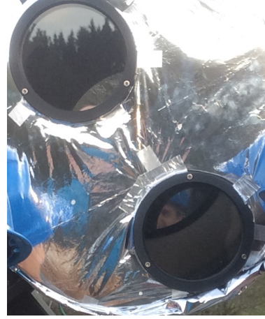
(b) DIMM mask at the entrance of the telescope tube.
