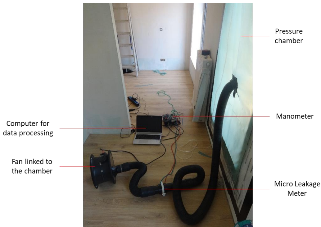
Figure 5 – setup of the experiment in the measurement of newly-installed windows (class 4) on a masonry wall using loose pressure chamber
