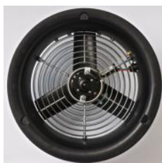
Figure 1 – Fan used to pressurize and depressurize the pressure chamber
