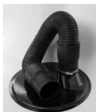
Figure 2 – flexible duct used to connect the fan to the pressure chamber
