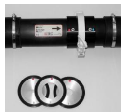
Figure 3 – “Micro Leakage Meter” for airflow measurement
