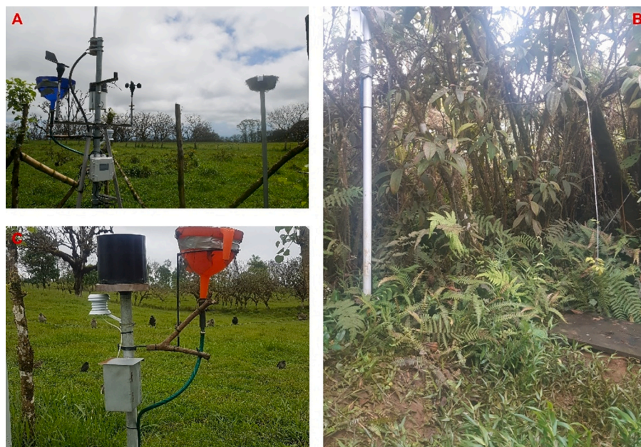
Fig. 2. View on the sites where the field equipment was installed. (A). Weather station located in the middle of the study area in a silvopastoral system (P450). (B). Pluviometer and air temperature/relative humidity probes installed in the at-risk silvopastoral system with conservation of trees and living fences (P420) and (C). View on the vegetation in the forest remnants where the soil frequency capacitance probes (METER TEROS12) are installed at 50 cm depth in the forest soil (FOR1).
