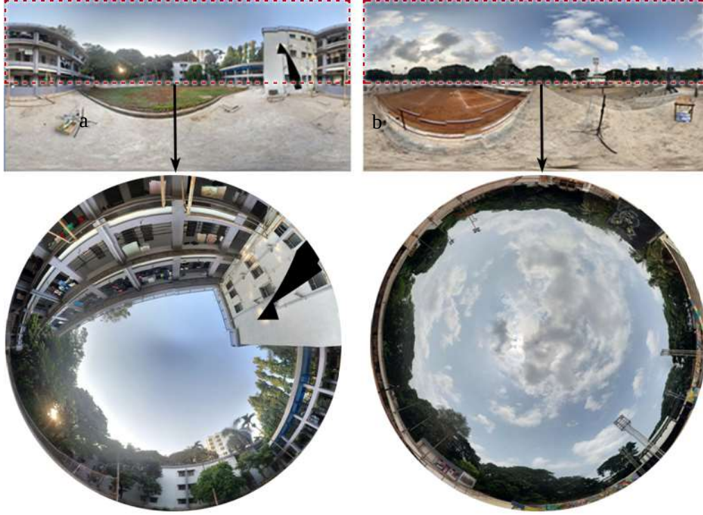
Figure 8: Generation of fisheye image through polar coordinate conversion for two tested locations: a) Urban Location: Hostel 1, IIT Bombay; and b) Sparse Location: Open Air Theater, Students Activity Center, IIT Bombay
