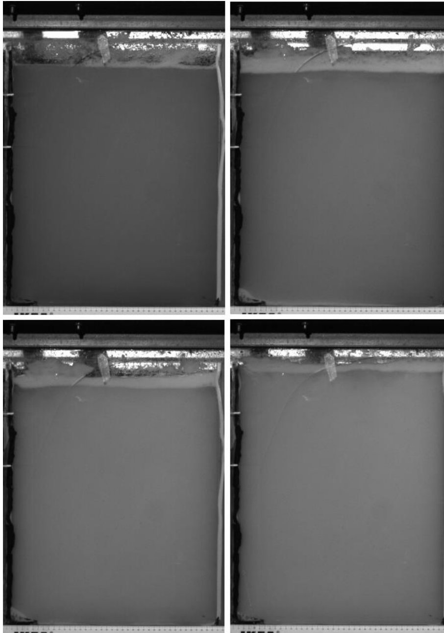
Figure 6.18. Reference images for kaolin clay concentration of 1%, 3%, 5% and 7%.
