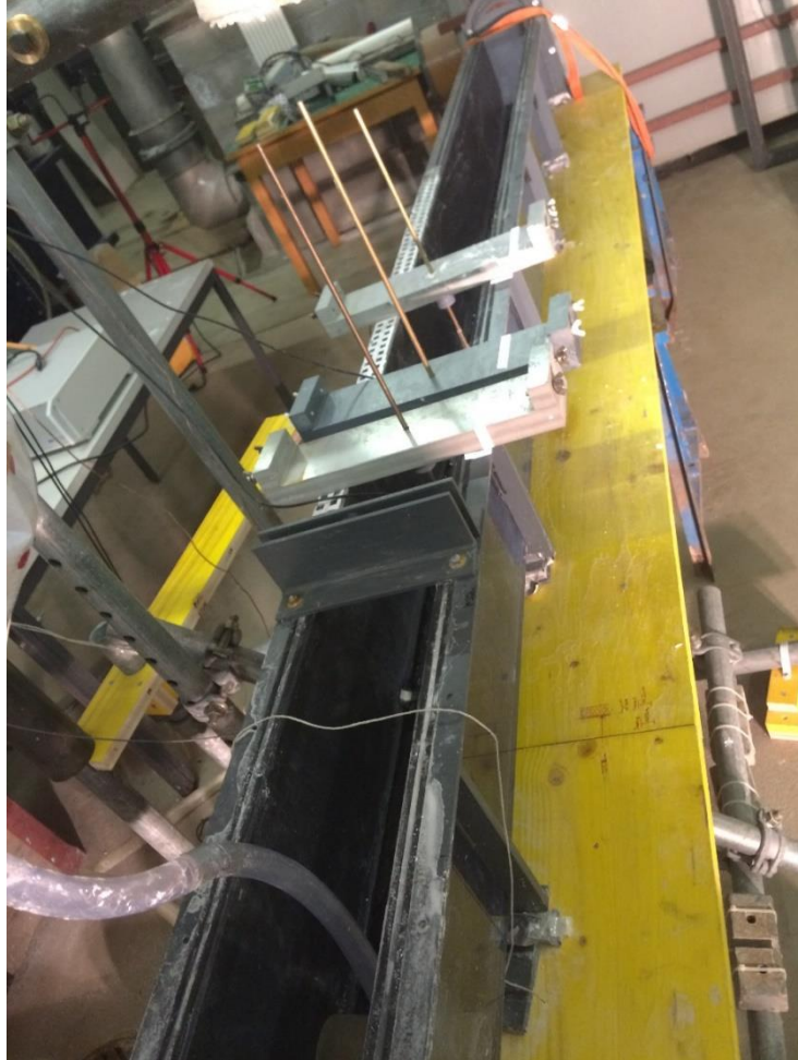
Figure 5.10. Pictures of the transducers placed in the flume.
