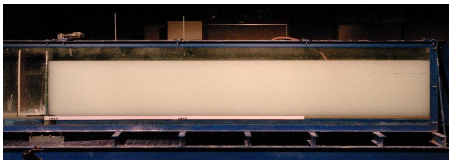
Figure 6.4. Example of reference image using water-milk mixture (captured by the digital camera).
