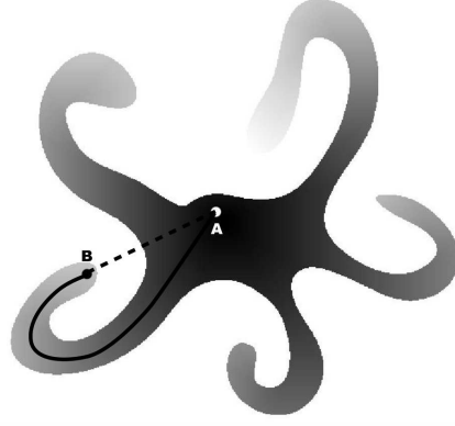
Figure 2.4: Geodesic distance map example. The geodesic distances with respect to point A of all region pixels are displayed in increasing grayscale value. Euclidean (dashed) and geodesic (solid line) distances from point A to point B are compared
