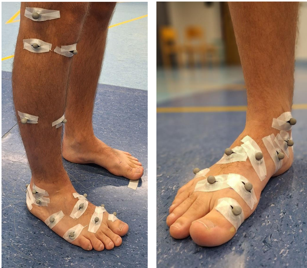
Figure 24. Marker placement according to Rizzoli multi-segment foot model. Lateral view (left image) and medial view (right image).
