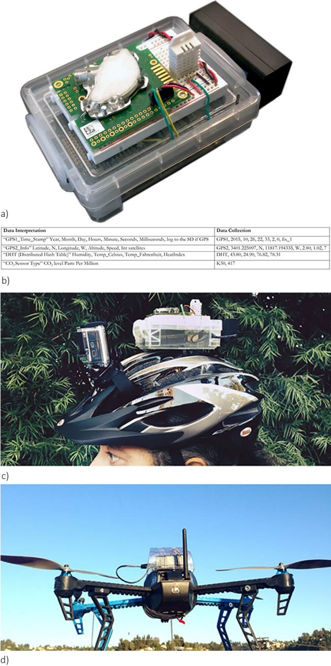
Figure 1: a) Portable sensor kit (Humidity/Temperature + CO 2 sensors with GPS shield and microcontroller). b) An instance of collected data on the University of Southern California campus. c) Custom air quality sensing kits are mounted to bike helmets for horizontal sensing. d) Custom air quality sensing kits attached to Unmanned Aerial Vehicle (UAVs) for vertical sensing.
