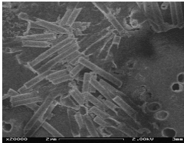
Figure 7.3: Ni NTs of diameter 150 nm released from PC templates.
