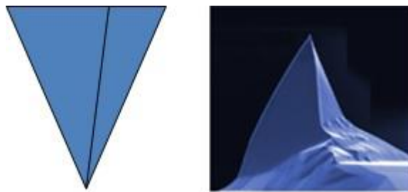
Figure 3.22: The schematic (left) and SEM image (right) of a MESP-HM tip from Bruker®.
