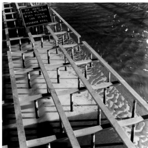
Figure 2.11: Overbank deposition of 0.1mm sediment in suspension in the FCF Wallingford (Knight et al., 1999)
