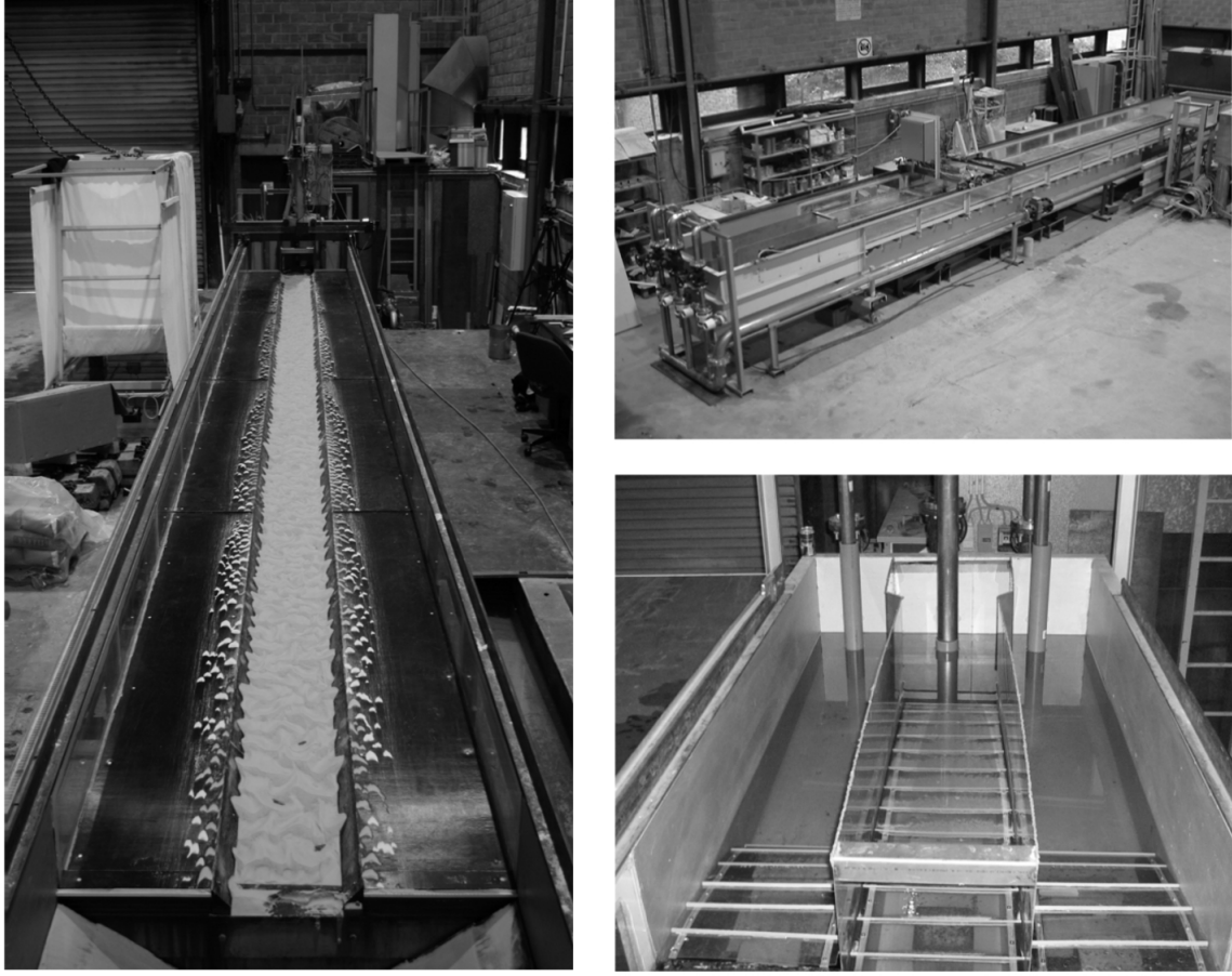
Figure 4.1: UCL compound channel flume. (Left) Compound channel with mobile bed experiment featuring bedforms, floodplain deposition and sand traps. (Upper right) General view with upstream discharge separation. (Down right) Upstream subsection separation and elliptical profiles
