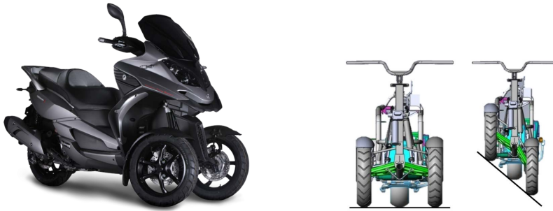
Figure 2.23: Quadro QV3 and its front suspension [162, 146].
