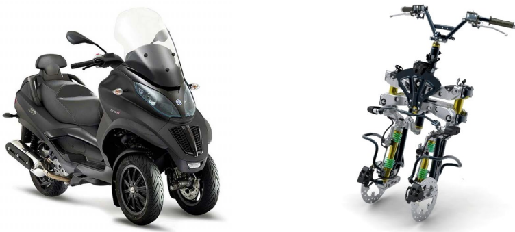
Figure 2.21: Piaggio MP3 500 Sport and its front suspension [159, 160].
