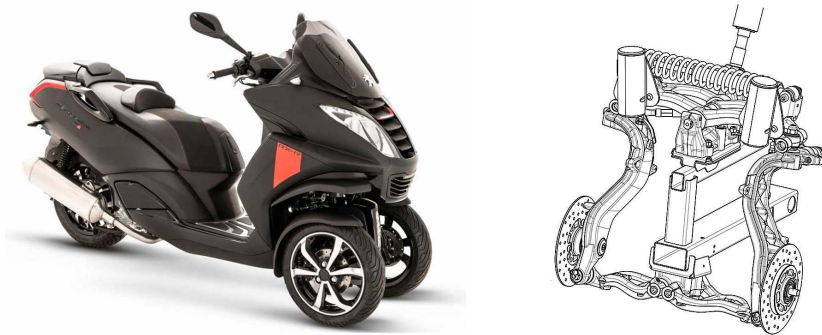
Figure 2.22: Peugeot Metropolis 400 RX-R and its front suspension [157, 156].
