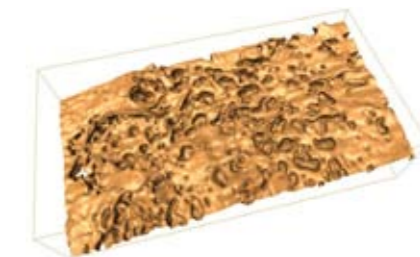
Figure 6: Juilland [2009] FIB reconstruction of an alite surface hydrated in paste for 7 hours. Dimension of the box: 1.75µm x 1µm x 400nm
