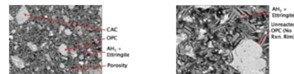
Figure 1: Formation of "ettringite" type microstructure after 1 day of hydration.
