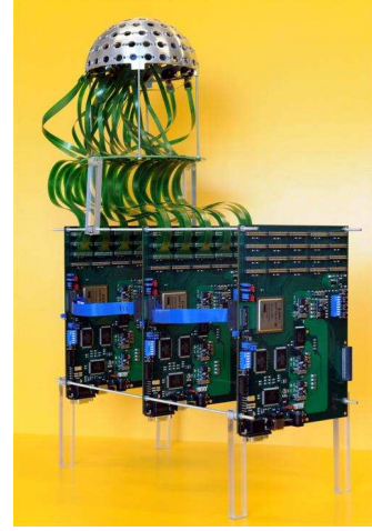
Figure 18: The setup of the FPGA platform for the 7-floor Panoptic system with thirty embedded cameras
