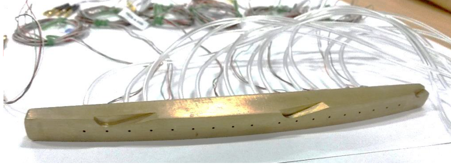
Figure 2.19: Instrumented pressure insert - hub endwall plane 02
