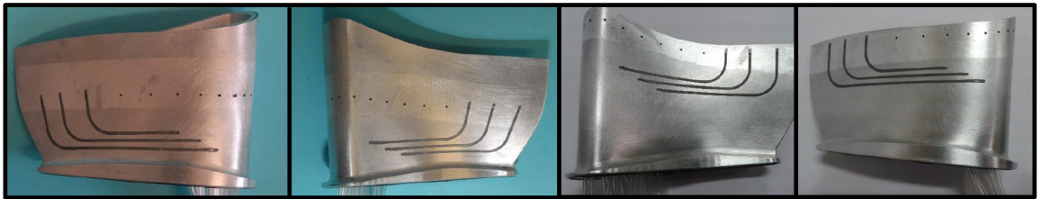
Figure 2.18: Vanes instrumented with static pressure taps at 50% span (a) and 90% span (b)
