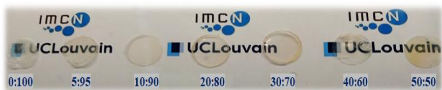
Figure 5.2.1: Images of CSBO:PEO (y:z) SPEs with 20% wt LiTFSI.
