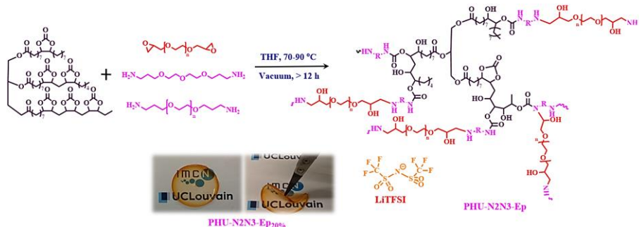
Scheme 6.2.2: Synthesis of mixed poly(hydroxyurethane)-poly(epoxy) networks with PEGDCE, (bottom-right: picture of PHU-N2N3-Ep films (75 mol% of N2, 25 mol% of N3 and 100 wt% of poly(epoxy) with respect to CBSO)), subscript indicates x-wt% LiTFSI).
