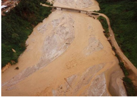
Figure 1.1: Massive aggradation of Ok Tedi river at Tabubil in mountain area after a landslide, 1984 http://www.rettet-die-lbe.de/oktedi/environ2.htm
