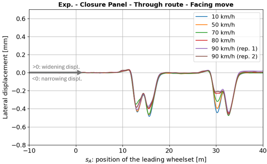
Fig. 6.8 Facing move: displacement of the external rail measured by the LVDT sensor during train passage on the through route. Negative values indicate movement inwards toward the center of the track.
