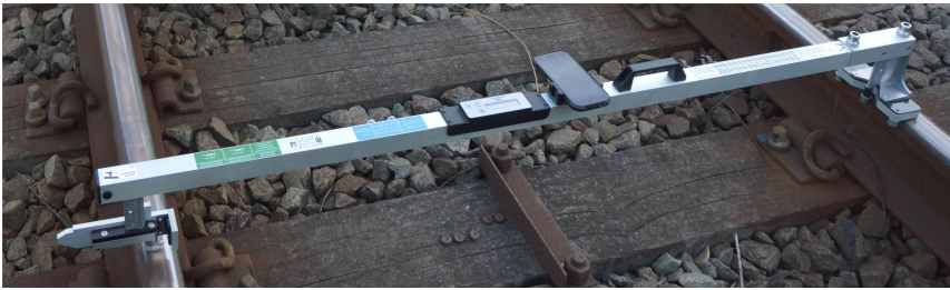
Fig. 3.4 The digital ruler [79] is used for static measurements of a railway track.
