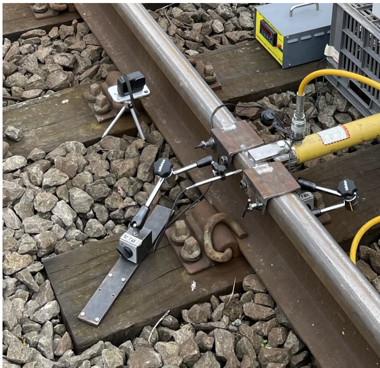
Fig. 4.3 Experimental setup showing the hydraulic jack coupled to the rail, with two U-shaped pieces securing the assembly longitudinally and the LVDT sensor positioned to measure rail displacement.
