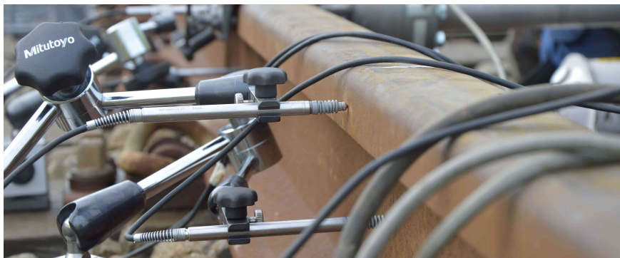
Fig. 3.5 LVDT were placed in different S&C zones to measure the rail head lateral displacement and rail web flexion.
