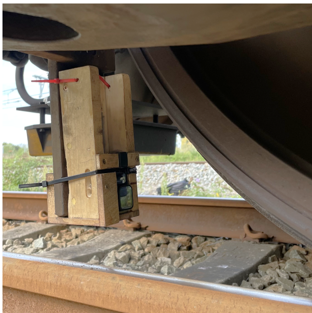
(a) GoPro camera with its mounting system
