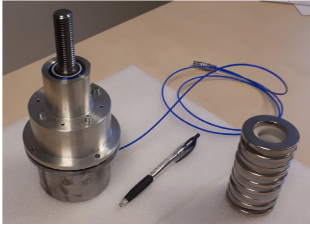
Figure 2.10: On the left side, the test bench and on the right side the PM rings.
