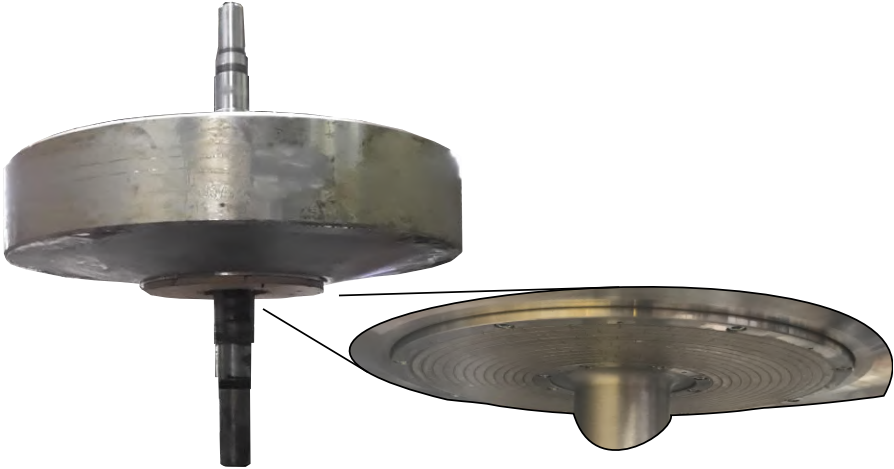
Figure 4.22: Rotating part of the PMTB placed on the flywheel system.
