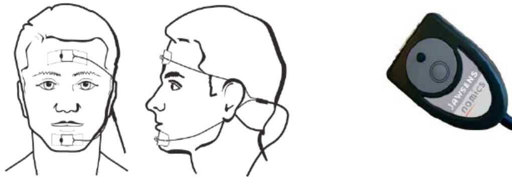
Fig. (1). Mandible movement sensor. The probes are placed on the median line of the face on the forehead and on the chin. The mandible movement signal corresponds to the distance between them. The Jawsens device that interfaces the sensor to the PSG system is illustrated on the right.
