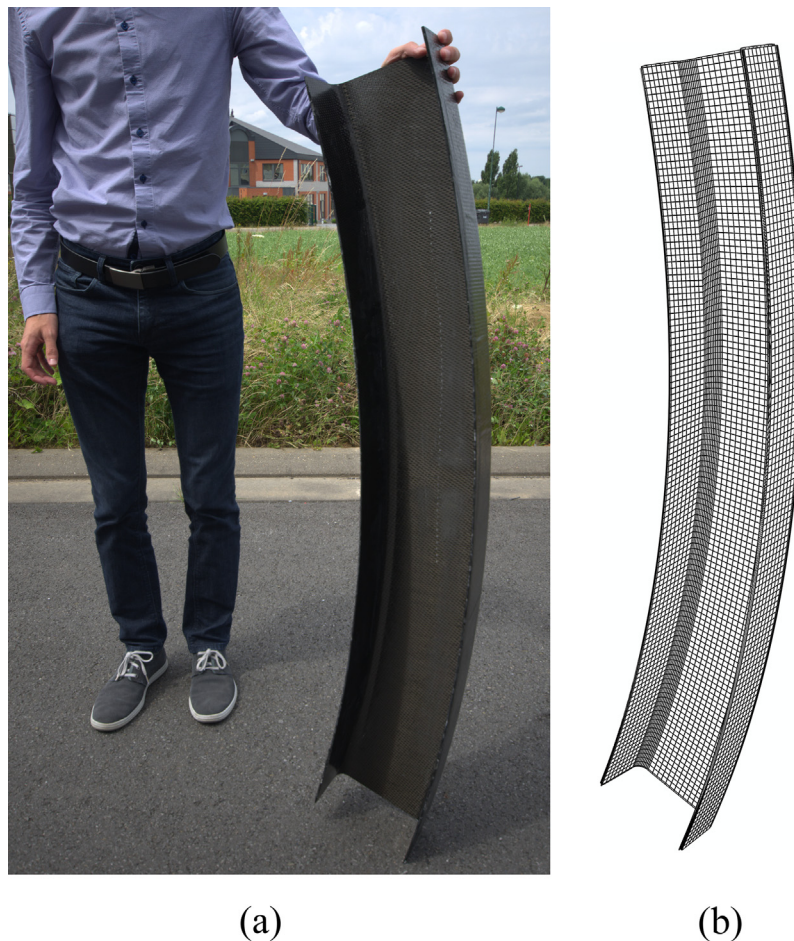
Fig. 5. (a) Picture of a manufactured C-spar and (b) typical volume mesh used for the FE prediction of the distortions of the C-spar. The part is meshed with twelve elements through the thickness, i.e. one element per ply.
