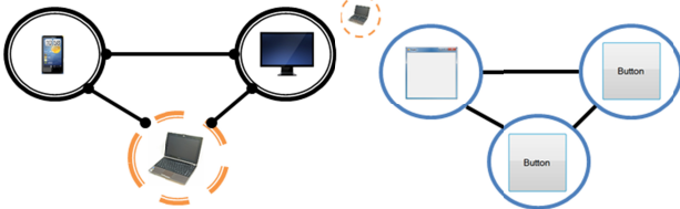
Figure 2. A distribution scene made up of: a cluster of three platforms (a) and an associated graph of CUI models (b).
