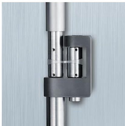
Figure 5.1: Extensional viscosity fixture consists of a fixed and rotating drum, which winds up the sample at constant Hencky strain rate, while measuring the force generated in the sample. Since the torque measurement is decoupled from the motor, no bearing friction correction is required. The picture is adapted from http://www.tainstruments.com/ .
