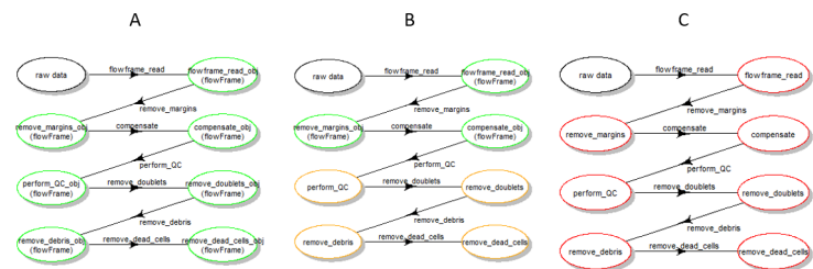
Figure S2. Illustration of the colour code used to represent the pipeline workflows. Green steps are the ones that have already been run and produced results, indicating a non problematic run. Orange steps are the ones that are correctly defined, but have not run yet for the displayed sample file. Red steps show an inconsistency problem between the already stored results, and the CytoPipeline object, meaning that the pipeline was previously run, either with a different number of steps, or with one or several steps that used a different method or different set of parameters. On the above picture, part A shows a situation where part of the pipeline has fully run. Part B shows a situation of pipeline that has run, but not all steps. Part C shows an inconsistency between the pipeline definition and the results stored.
