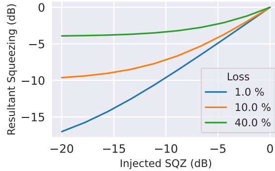
Figure 2.8: Achievable squeezing for a given squeezing injection and loss. Reproduced from Ref. [2].
