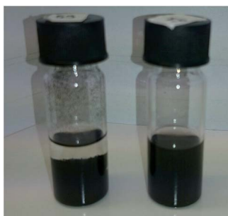
Figure 5.4 – Suspensions ( 0.5 \text{ mg} \cdot \text{mL}^{-1} ) in \text{CH}_2\text{Cl}_2 . On the left side: MWCNT-initiator after 5 min rest; on the right: MWCNT- g -PTMPM after 24 h rest.
