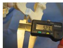
Fig. 5 : Maximal gap between host and graft was measured with an electronic caliper.
