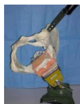
Fig. 2 : Sawbone was rigidly fixed by a steel clamp with a 360° - rotational base. Cutting was performed using an oscillating saw.
