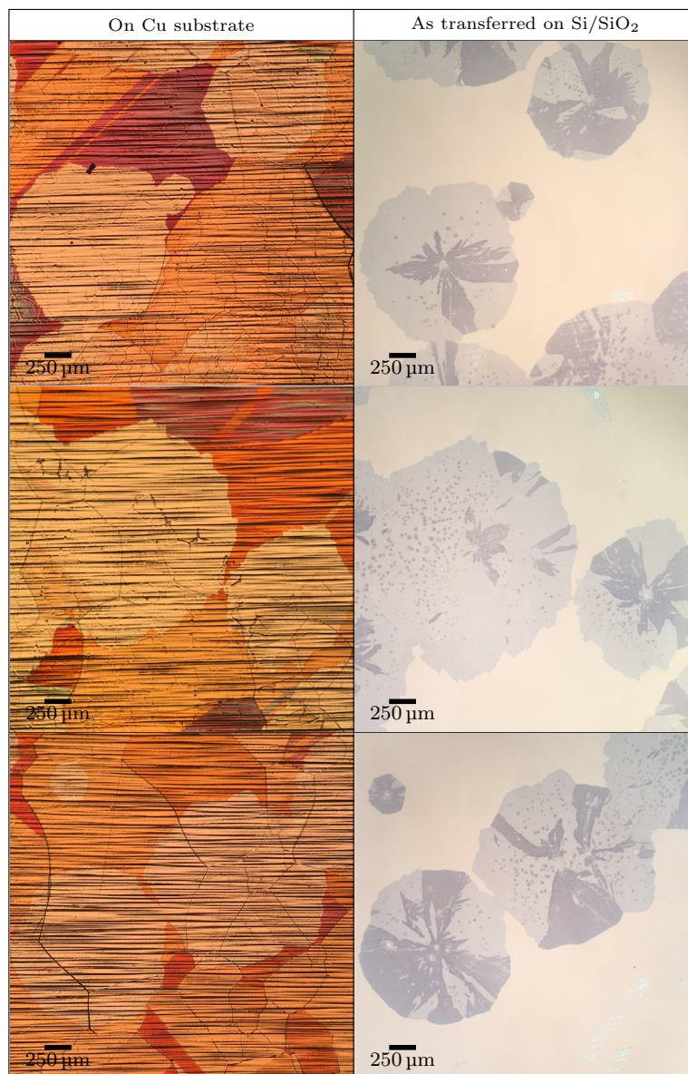
Figure 7.12: Optical microscope images taken before (left panel) and after the transfer process (right panel). Left panel shows the Cu surface underlying the graphene domains while the right panel shows the graphene additional layers.
