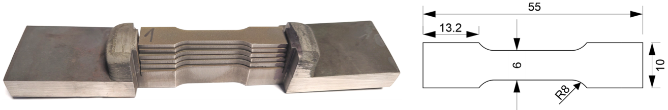
Fig. 1 (a) Tensile specimens extracted from L-DED fabricated cuboids by means of wire cutting, (b) dimensions of the samples.
