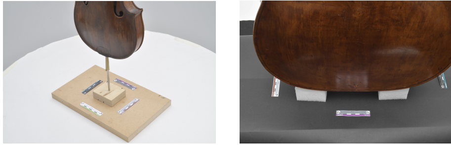
Fig. 2: Four scale bars are used during the data acquisition process. Examples for a violin (left) and a cello (right)
