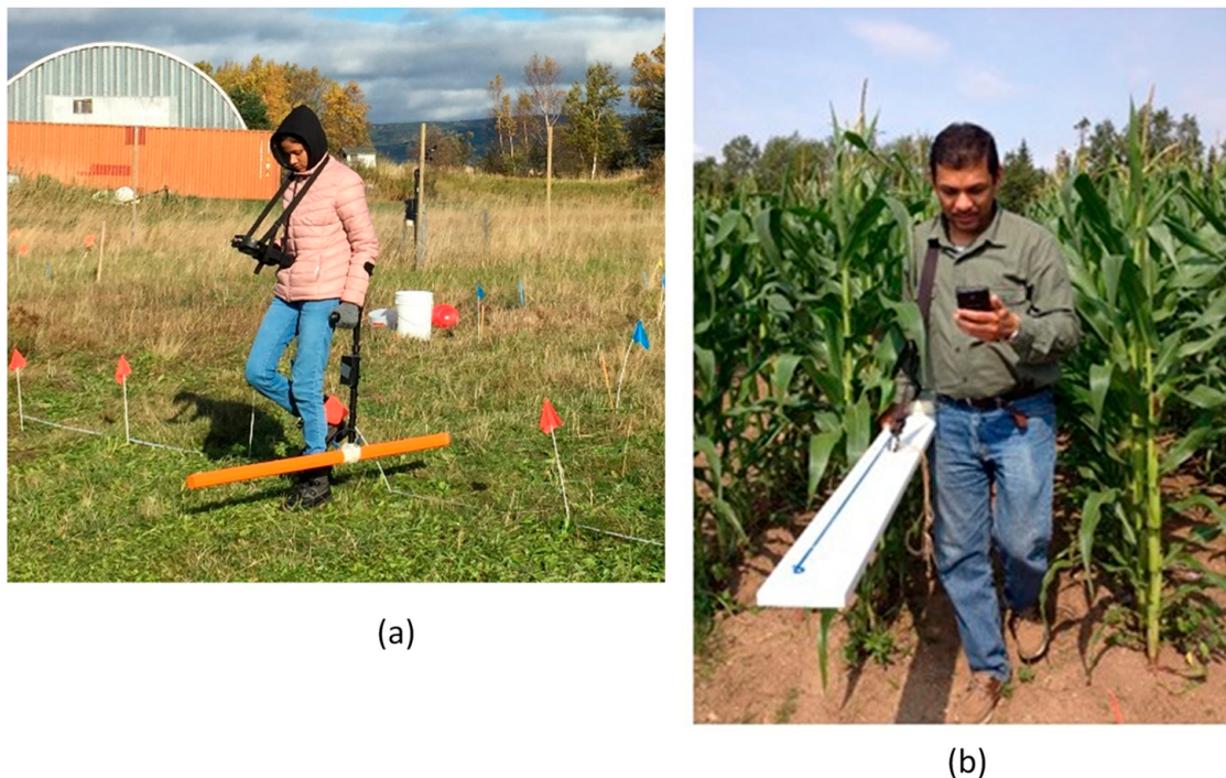
Figure 7. Electromagnetic induction (EMI) surveys with (a) multi-coil EMI sensor (CMD-MINIEXPLORER) (EMI instrument by S. Pathirana) and (b) multi-frequency EMI sensor (GEM-2) (EMI instrument by L. Galagedara).
