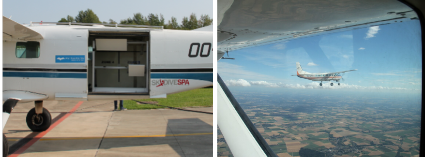
Figure 2.3: (left) MetaSensing BV's airborne L-band SAR system on-board one of the two CESNA Gran Caravan airplanes and (right) a picture of one airplane taken from the other while flying in the across-track (XT) configuration.
