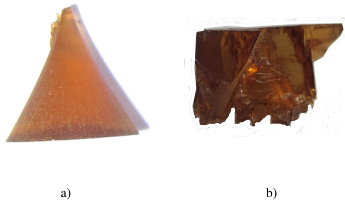
Figure 12: Uniaxial compression: fragments after failure: a) typical conical fragment with rough fracture surface, b) typical other fragment with essentially mirror-like fracture surfaces.
