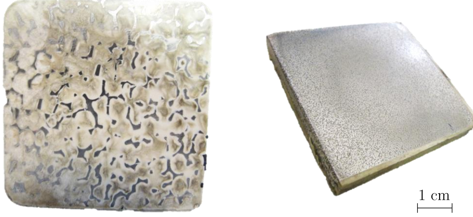
Figure 6.5: Pictures of two metallic foams infiltrated with polyester by hot uniaxial pressing. The metallic phase appears in grey, the polyester in yellow.
