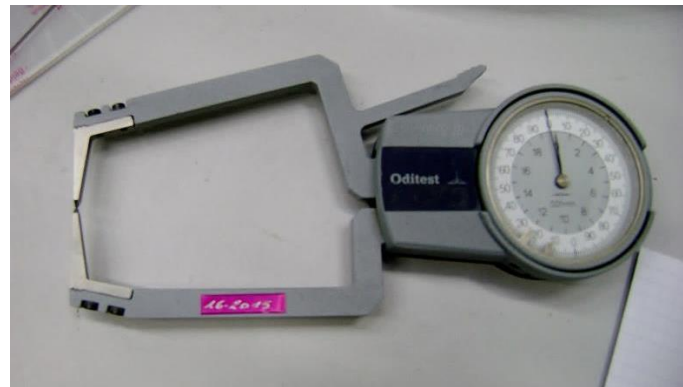
Figure 5.30: Picture of the caliper gauge used to measure the thickness of the erosion samples before and after the test.
