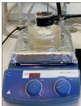
Fig. e.2 - Wet impregnation (WI) setup for supported catalysts preparation.
