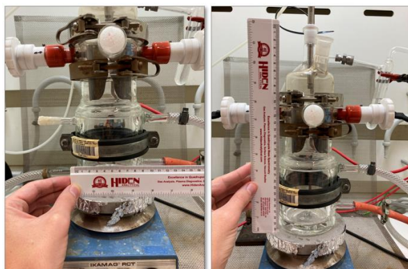
Fig. e.4 - Glidarc plasma (GP) setup in batch configuration, showing the glass reactor diameter (left) and its height (right).
