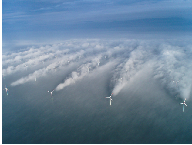
Figure 1.2 – Aerial view from the Southeast of wake clouds at Horns Rev on February 12, 2008 (© Vattenfall, Horns Rev 1 owned by Vattenfall. Photographer Christian Steiness).
