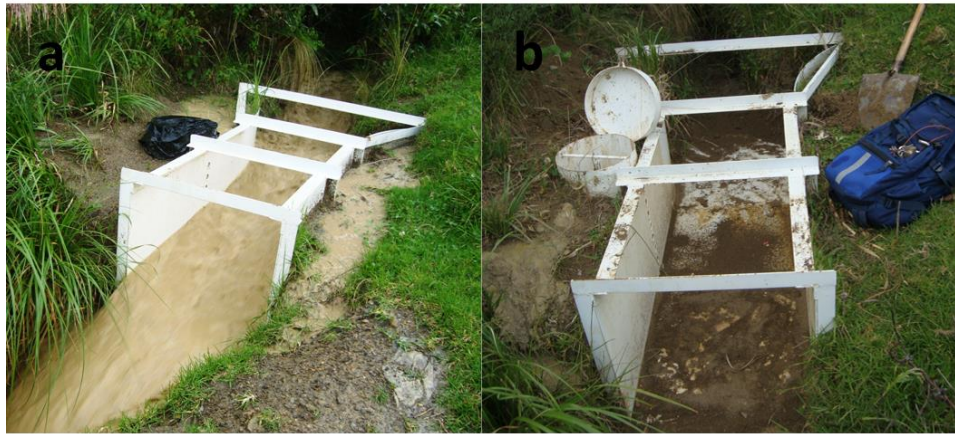
Figure 41: Flume in AI micro-catchment: a) during and b) after an event.
