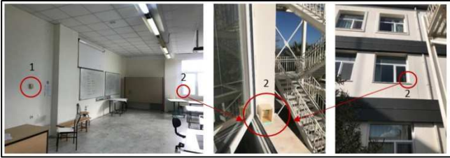
Fig. 2. Photos of inner and outer climate data loggers (1: indoor, 2: outdoor).
